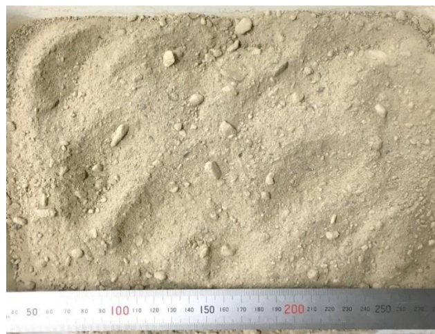
Figure.3.4 Komaoka volcanic coarse grained soil
