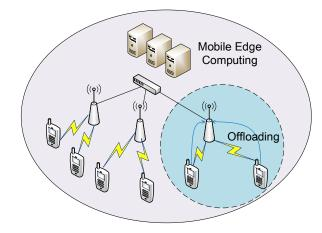
Fig. 1. A multi-user mobile-edge computing system
