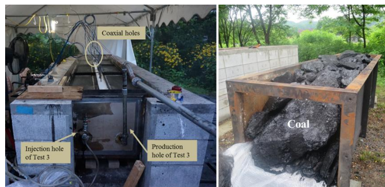
Fig. 2. Construction of UCG model.
