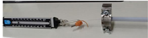
Fig. 5. Control method for braid tension.
