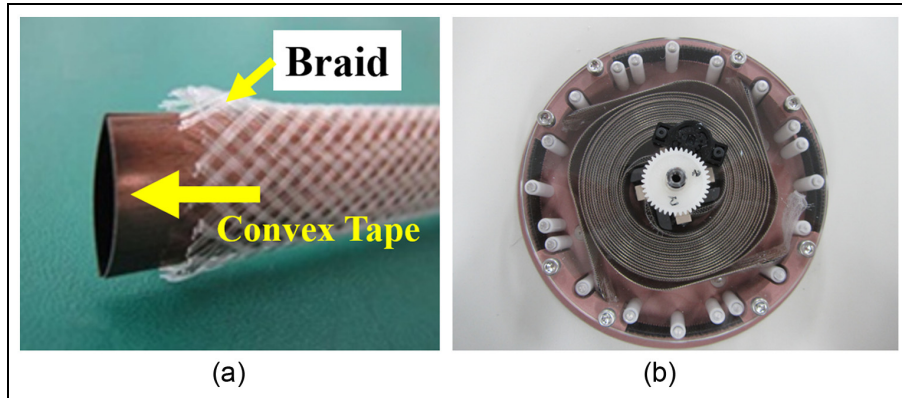
Figure 1. Schematic photo of BCON boom and stored configuration: (a) BCON boom configuration and (b) packed configuration of four BCON booms.
