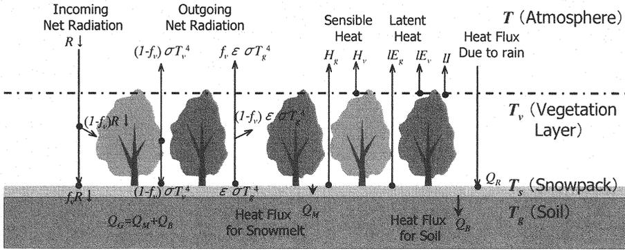
Fig. 3. Schematic figure of the two-layer model
