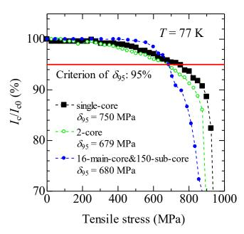
Fig. 4. Critical current ratio  $I_c/I_{c0}$  under tensile stress. The criterion for tensile stress tolerance was 95% of  $I_{c0}$ .
