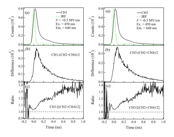
Figure 5. (a) PL decay profile observed at 640 nm in the presence of +0.3 MVcm<sup>-1</sup>, i.e., CH1 (left) and -0.3 MVcm<sup>-1</sup>, i.e., CH3 (right), (b) difference between CH1 and (CH2+CH4)/2 (left) and between CH3 and (CH2+CH4)/2 (right), and (c) ratio between CH1 and (CH2+CH4)/2 (left) and between CH3 and (CH2+CH4)/2 (right). Note that (CH2+CH4)/2 corresponds to the decay at zero field.
