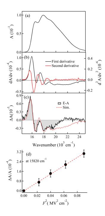
Fig. 2. Absorption spectrum of P3HT dispersed in a PMMA matrix (a), the first and the second derivatives of the absorption spectrum (b), E-A spectrum observed with a field strength of 0.3 MVcm<sup>-1</sup> (c), and plots of the field-induced change in absorption intensity at 15820 cm<sup>-1</sup> (d). In (c), the black line shows the observed spectrum, and the red line shows the simulated spectrum.
