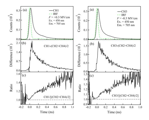
Figure 6. (a) PL decay profile observed at 705 nm in the presence of +0.3 MVcm<sup>-1</sup>, i.e., CH1 (left) and -0.3 MVcm<sup>-1</sup>, i.e., CH3 (right), (b) difference between CH1 and (CH2+CH4)/2 (left) and between CH3 and (CH2+CH4)/2 (right), and (c) ratio between CH1 and (CH2+CH4)/2 (left) and between CH3 and (CH2+CH4)/2 (right). Note that (CH2+CH4)/2 corresponds to the decay at zero field.
