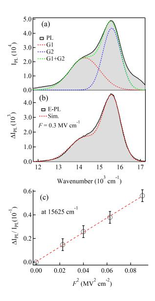
Fig. 3. PL and E-PL spectra with excitation at 450 nm. (a) PL spectrum and the decomposition to the G1 and G2 bands, which were used for the simulation of the E-PL spectrum. (b) E-PL spectrum observed with a field strength of 0.3 MVcm<sup>-1</sup> (black solid line), and the simulated spectrum (red broken line). (c) Plots of  $\Delta I_{PL}/I_{PL}$  as a function of the square of applied field strength. E-PL spectrum was monitored at the second harmonic of the modulation frequency.
