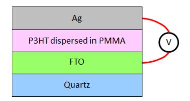
Fig. 1. Layer structure of the device used in the present work. FTO and Ag films were used as electrodes to apply external voltages (V) to the P3HT dispersed in a PMMA matrix.
