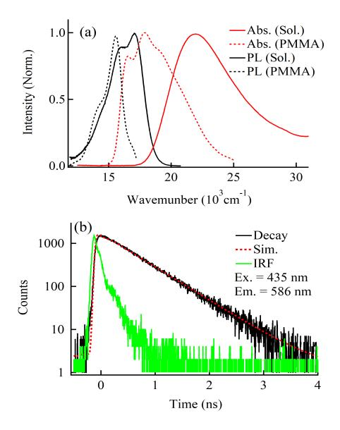
Fig. 4. (a) Absorption spectra (red line) and PL spectra (black line) of P3HT in solution (solid line) and P3HT distributed in a PMMA matrix (broken line). (b) PL decay profile in solution (black line) observed at 586 nm with excitation at 435 nm, the instrumental response function (IRF) (green line), and the decay simulated by assuming a single exponential function (red line). PL spectra in (a) were obtained with excitation at 450 nm.
