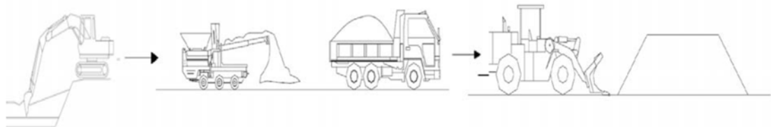
Figure 2.5 Placement of cement treated soil along slope (Tang et al., 2001)
