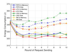
Fig. 3. Total Energy Consumption of Edge Caching in TTL of Caching Time (TCT)
