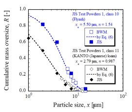
Fig. 3 Particle size distributions of JIS Test Powders 1, class 10 (Flyash) and class 11 (KANTO (Japanese) loam)
