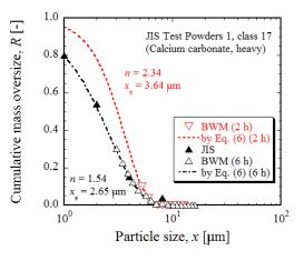
Fig. 4 Particle size distributions of JIS Test Powders 1, class 17(Calcium carbonate, heavy)
